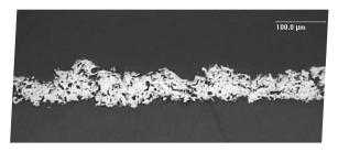
Spondycoat<sup>®</sup>-T 371A is a Titanium coating with low roughness (representative values of Ra 4-10  $\mu$ m) mainly indicated for thin layers (recommended thickness 60-120  $\mu$ m).
