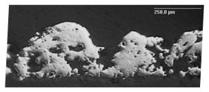
Ti-Growth<sup>®</sup> P is a porous Titanium coating with high roughness (representative values of Ra 40-80 μm) and a recommended thickness of 300-500 μm.
